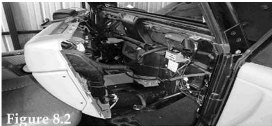
Figure 8.1 Drain Studs Vacuum line Heater hoses
