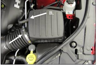
**2. A)** Loosen the hose clamp on the airbox side of the factory intake tube. **B)** Disconnect the crankcase breather line from the airbox lid.
