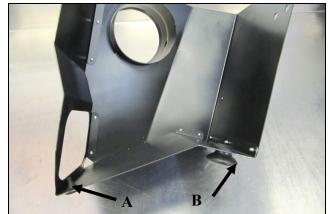
**9. A.)** Install the Rubber bumper (#12) into the small hole in the panel assembly.
