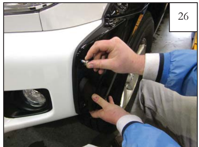
Slide a supplied .320 SS Washer (WA1-0012) onto a SS Torx Screw (SW1-0041). Situate flare on bumper, inserting screws through holes drilled in bumper in step 24.
