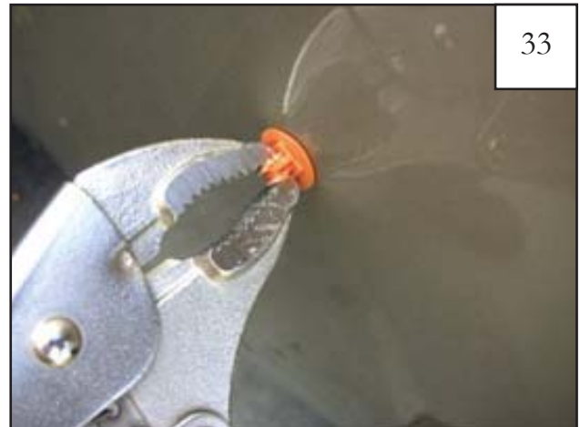
Remove three clips from fender using vise grips, pulling with a rocking motion. See step 34.
