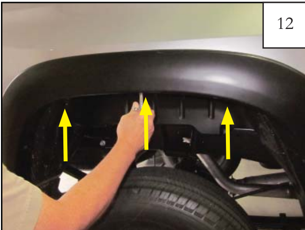
Hold the flare firmly on the fender. Start three supplied 20mm Hex Screws (SW1-0036) through the top center holes of the flare and into factory holes in fender.
