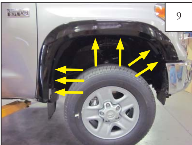
9 Ensure flare is properly positioned and tighten all screws. Installation Complete. (See steps 5-7)
