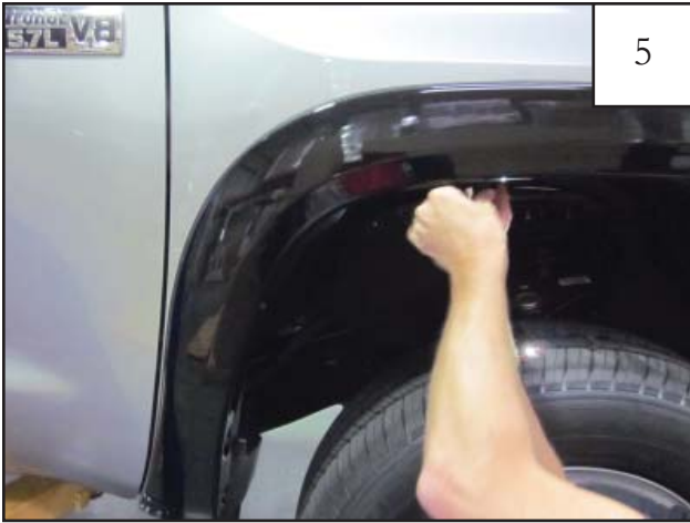
5 Place flare on fender, aligning holes with clips on the bracket. Start two supplied 20mm Hex Screws (SW1-0036) through two holes on the top of the flare and into clips.
