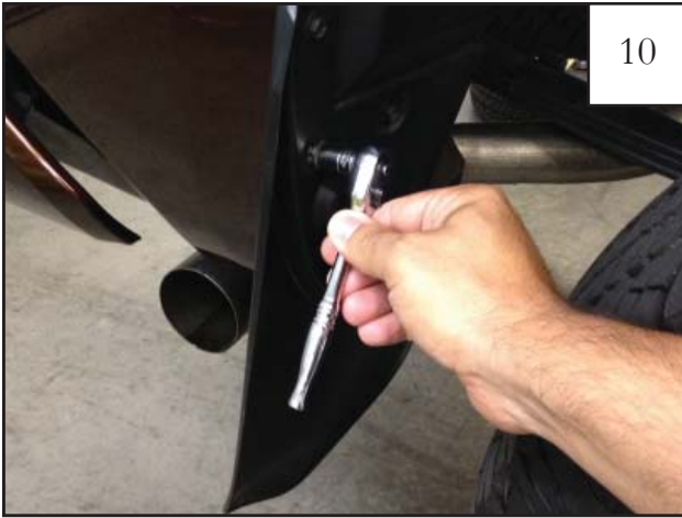
Using a socket wrench with a 10mm socket, factory screw second from the top of the mud guard.
