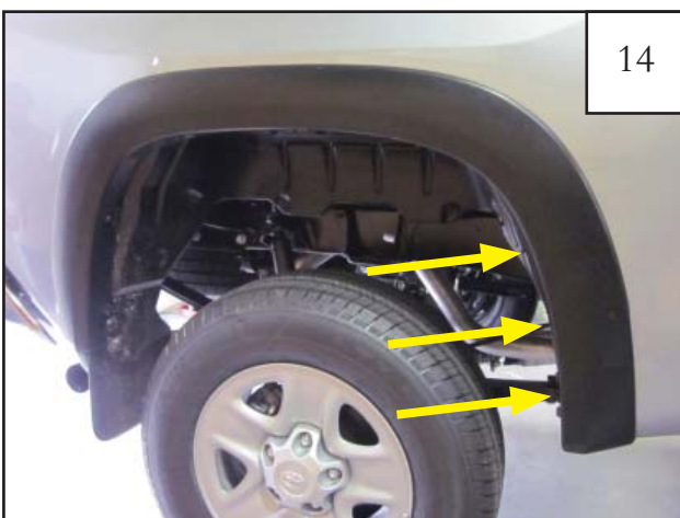
Using 10mm socket, start three supplied 20mm Hex Screws through the forward most holes of flare and into factory holes in fender.
