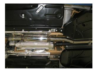
**Step 3.** Begin installation of your new MAGNAFLOW system by attaching the Resonator Assembly to the "Y" collector outlet using the supplied 2.50" clamp. Keep all fasteners and clamps loose until final adjustment.
