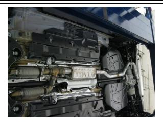
**Step 1.** Begin removal of the OEM exhaust system by loosening the clamp behind the "Y" collector.
