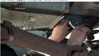
Reinstall the six transfer case skid plate bolts.
