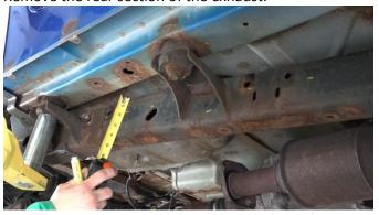
Mark down 1.5 inches from the top of the frame rail, on the inside and outside. You will do this from the front most body mount bracket to the bend at
