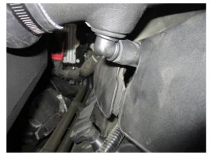
11. Attach the breather hose to the 3/4" elbow fitting in 12. Connect the ATS sensor wiring harness back the air duct.
