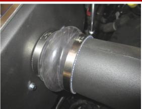
10. Locate the remaining #56 clamp and # 654 clamp. Slide the #64 clamp onto the hump hose and the #56 clamp onto the straight sleeve and install the CORSA air duct into the hump hose and straight sleeve. Adjust the air duct as necessary and fully tighten all four clamps using a flat head screwdriver or ratchet and 8mm socket.
