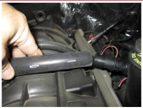
2. Locate the supplied 3/4" x 21" breather hose and install onto straight fitting. Install factory breather elbow back onto driver's side vent.
