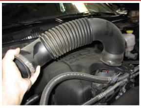
2. Loosen the clamps securing the factory air duct to the throttle body and factory air box using flathead screwdriver or ratchet with 8mm socket. Remove factory air duct from vehicle.
