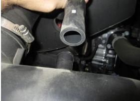
**3.** Disconnect factory breather hose from factory air box by pulling straight out.
