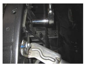
Remove the two 13mm air box mounting tray bolts securing the tray to the inner fender.
