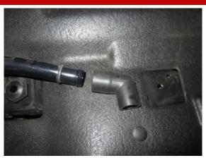
**6.** Remove the breather hose from the driver's side vent and remove the elbow from the breather hose.
