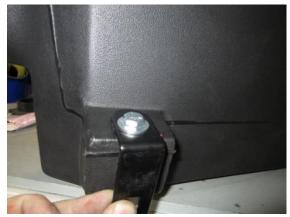
Locate the longer L-bracket, one 6mmx25mm bolt, flat washer, lock washer, and 6mm nut and install bracket to front side of box closest to headlight.
