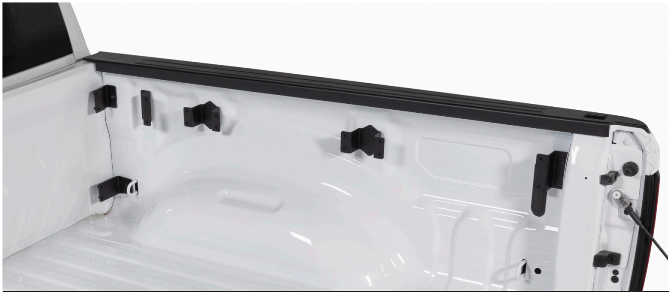
Light Duty Ram with All Brackets Installed
