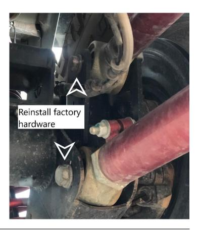
32. Rear Lower will used supplied 4" x 9/16" bolt, washers and small flag nut on both driver and passenger side frame. \*Rear Upper will used supplied 3.5" x 9/16" bolt, washer and small flag nut on both driver and passenger side frame.
