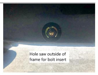
22. On rear, we need to trim some of the rear body mount bracket on frame just rearward of the body mount itself on driver/passenger sides. Use the EVO Long arm as a template and slowly trim and fit body mount bracket until bracket fits nicely against body mount bracket and lower hole on underside of frame line up to install bolt. Roughly the rear side of the body mount will need to be full trimmed and cleaned to frame ~1/2" rearward of body mount small bolt.
