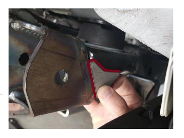
26. On rear axle, cleanly cut and grind smooth to axle tube the entire driver and passenger side rear lower control/shock mounts. Upper control arm mounts on axle will stay unmodified.
