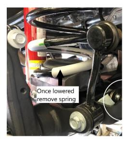
13. Remove upper control arms from frame and axle and set aside. Axle will be loose at this time use caution and appropriate support.
