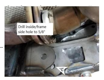
21. On outside of frame we need to make a relief hole to install nut and washer inside frame to newer lower control arm bolt. Using at 1" or larger hole saw and the previously drilled pilot hole make hole in OUTSIDE of frame ONLY.
