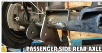
Once positioned, tack in place. Verify correct location of left and right and weld all connections to axle. Both sides.
